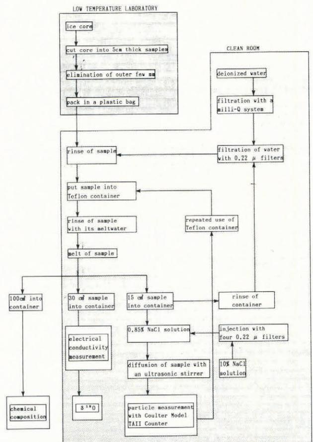
Fig.2. Processing of ice-core samples for microparticle counting and electrical conductivity measurement.
