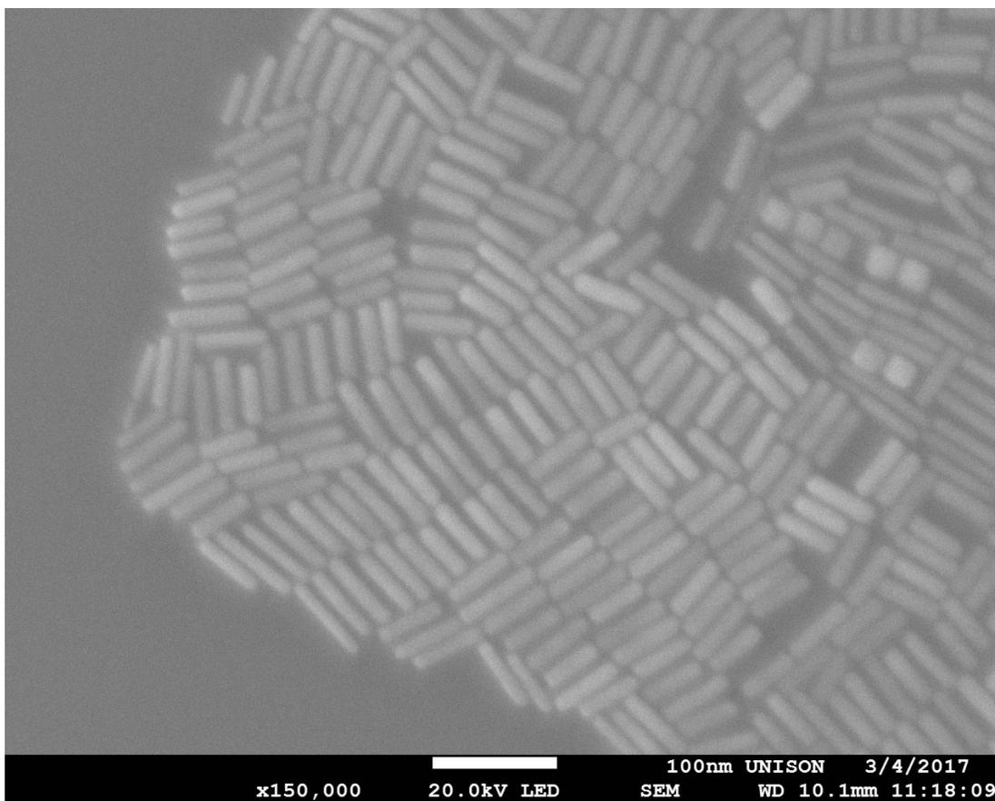
Figure 1. Figure 1. Scanning electron microscopy of gold nanorods
