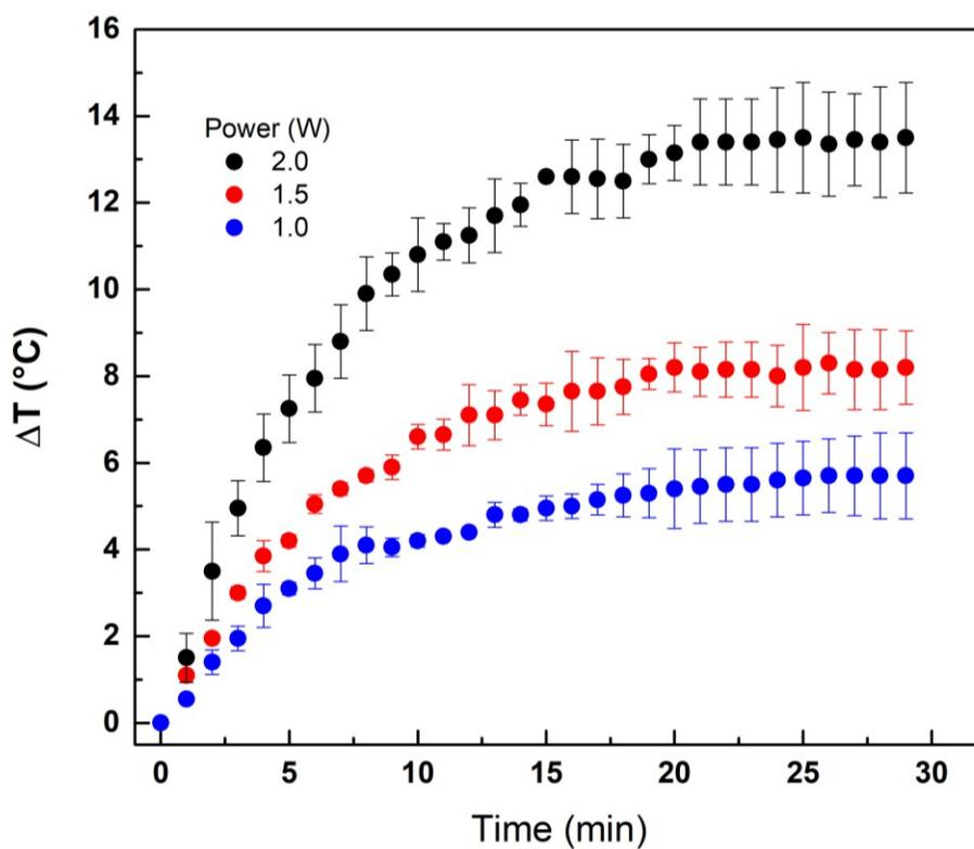
**Figure 2.** Figure 2. Heating tests for gold nanorods samples, irradiated with an 808 nm diode laser.
