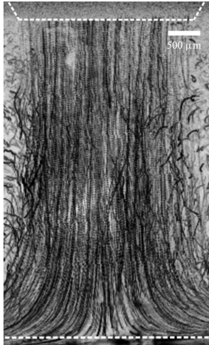
Figure 16. Side view showing the pathlines obtained from microscopic particles seeded into the wall jet flow and recorded with a high-speed camera. The top lines indicate the nozzle exit and the bottom line the position of the wall, v_{jet} = 5 \text{ m s}^{-1} .
