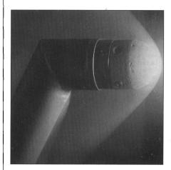
**ON THE COVER**: Test using high-temperature gas flow to evaluate a hemispherical functionally gradient material. From M. Koizumi and M. Niino in this issue, p. 20. For more information on functionally gradient materials, please see the section that begins on page 14.
