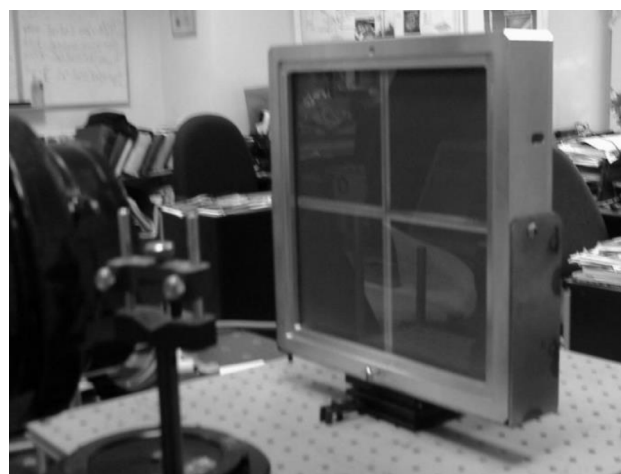
Figure 3. Photo of the bimorph deformable mirror 260 mm \times 260 mm attached in its mounting.
