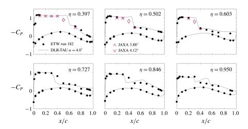
FIGURE 5. Surface pressure coefficient  $C_p$  at M = 0.85,  $Re = 5.0 \times 10^6$  and  $\alpha = 4.0^\circ$  comparing experiment and simulation at the six outermost spanwise stations.
