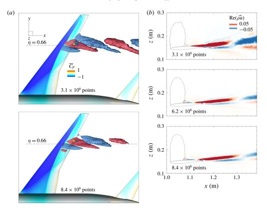
FIGURE 18. Mesh refinement for rightmost eigenmode showing (a) volumetric isosurfaces at two values ( $\pm 0.02$ ) of the x-momentum component  $\rho u$  for coarsest and finest mesh (see figure 7(b) for medium mesh) and (b) real part of x-momentum at constant spanwise station  $\eta = 0.660$ . Eigenvectors have been scaled by their respective maximum value in x-momentum, indicated by the yellow spheres, to compare results on different meshes.
