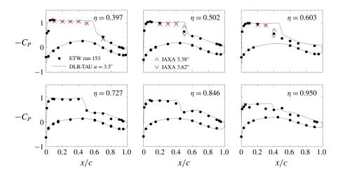
FIGURE 4. Surface pressure coefficient  $C_p$  at M = 0.85,  $Re = 5.0 \times 10^6$  and  $\alpha = 3.5^{\circ}$  comparing experiment and simulation at the six outermost spanwise stations.
