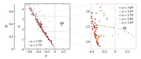
FIGURE 6. Computed eigenvalues for angles of attack between  $\alpha = 3.50^{\circ}$  and  $3.85^{\circ}$  showing Strouhal number *St* and angular frequency  $\omega$  over growth/decay rate  $\sigma$ . The three-dimensional shock-buffet mode with eigenvalue ( $\sigma$ ,  $\omega$ ) = (0.156, 2.371) at  $\alpha = 3.75^{\circ}$  is labelled SB.
