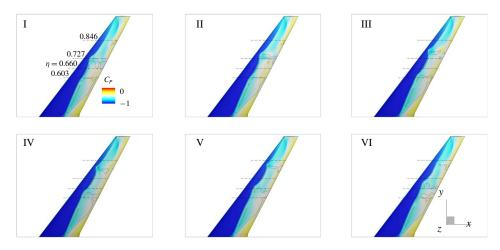
FIGURE 16. Time evolution of surface pressure coefficient,  $C_p$ , at six time steps during one fundamental, nonlinearly saturated oscillation cycle; cf. figure 14(e,f). Instantaneous reverse-flow regions are indicated by the dark grey zero-skin-friction lines.
