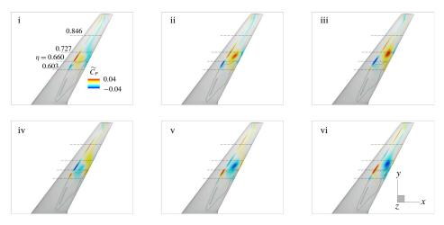
FIGURE 15. Time evolution of unstable eigenmode showing disturbance in surface pressure coefficient,  $\tilde{C}_p = C_p - \bar{C}_p$ , at six time steps during one oscillation cycle; cf. figure 14(*d*). Instantaneous reverse-flow regions are indicated by the dark grey zero-skin-friction lines.
