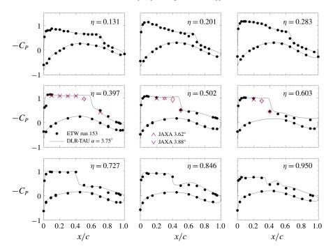
FIGURE 3. Surface pressure coefficient  $C_p$  at M = 0.85,  $Re = 5.0 \times 10^6$  and  $\alpha = 3.75^\circ$  comparing experiment and simulation along nine non-dimensional spanwise stations  $\eta$ . Streamwise coordinate x (measured from leading edge) is normalised by the respective local chord length c.
