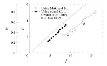
FIGURE 12. Angular frequency (and Strouhal number) as a function of spanwise wavenumber  $\beta$  for characteristic medium-frequency band of eigenmodes. Results are made dimensionless using either mean aerodynamic chord (MAC) and free-stream speed  $U_{\infty}$  or, when defining a plane approximately normal to the quarter-chord line, local chord  $c_n$  at the location of coherent cellular structures and velocity  $U_{\infty,n}$ . Labelling of individual modes follows figure 11.
