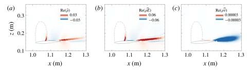
FIGURE 9. Slice at constant spanwise station  $\eta = 0.660$  showing real part of eigenvector's scalar quantities with density  $\hat{\rho}(a)$ , total energy  $\hat{\rho E}(b)$  and turbulence-field variable  $\hat{\rho v}(c)$ . The sonic line is highlighted by a dash-dotted line.
