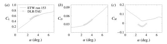
FIGURE 2. Aerodynamic loads at M = 0.85 and  $Re = 5.0 \times 10^6$  comparing experiment and simulation for (a) lift coefficient, (b) drag coefficient and (c) pitching moment coefficient.
