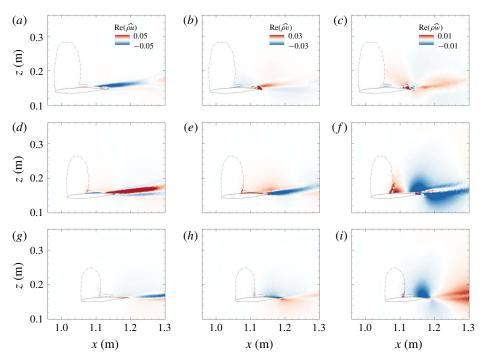
FIGURE 8. Slices at constant spanwise stations  $\eta = 0.603$  (a-c),  $\eta = 0.660$  (d-f) and  $\eta = 0.727$  (g-i) showing real part of eigenvector's momentum components with x-momentum  $\widehat{\rho u}$  (a,d,g), y-momentum  $\widehat{\rho v}$  (b,e,h) and z-momentum  $\widehat{\rho w}$  (c,f,i). The sonic line is highlighted by a dash-dotted line.
