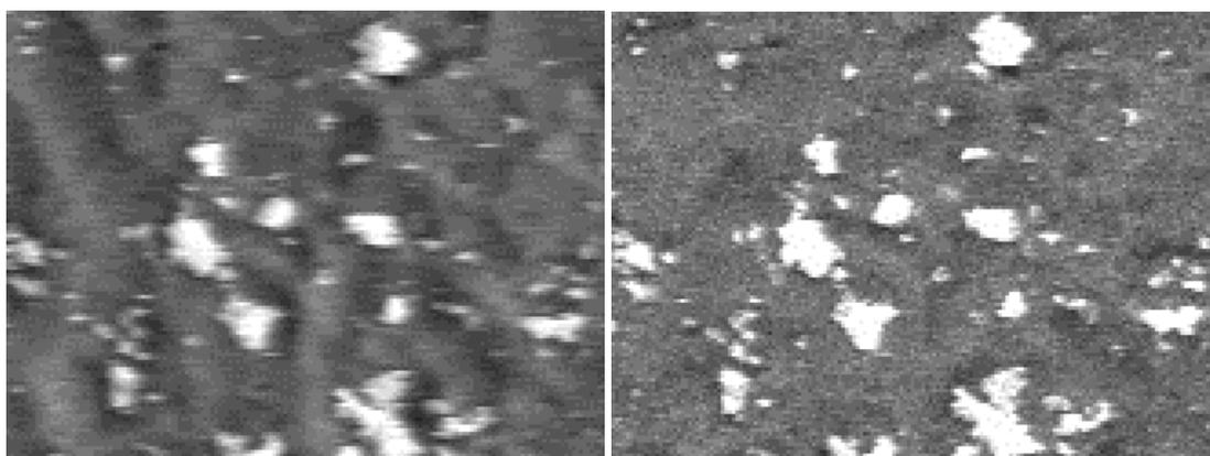
Fig.3. Comparison of two BSE image sections with 168 x 125 pixels taken at 100 nsec pixel dwell time. The left image was acquired with a conventional BSE detector with 250 nsec signal rise time and shows smearing in the scanning direction. The right image was taken with 80 nsec signal rise time and shows sharp details without smearing.
