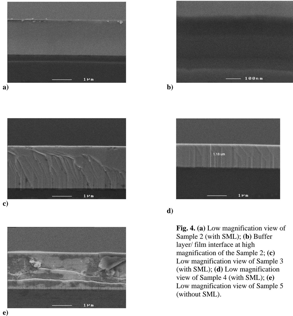
**Fig. 4.** (a) Low magnification view of Sample 2 (with SML); (b) Buffer layer/ film interface at high magnification of the Sample 2; (c) Low magnification view of Sample 3 (with SML); (d) Low magnification view of Sample 4 (with SML); (e) Low magnification view of Sample 5 (without SML).
