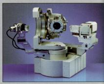
With the Philips X'Pert x-ray diffractometer line, you'll find a solution to even the most complex materials identification problems. X'Pert-MRD for advanced research, X'Pert MPD for powder diffraction, stress/texture, microstructure and crystallographic studies.
