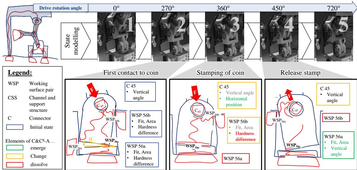
Figure 6. C&C<sup>2</sup>-Sequence model of the coinage machine
