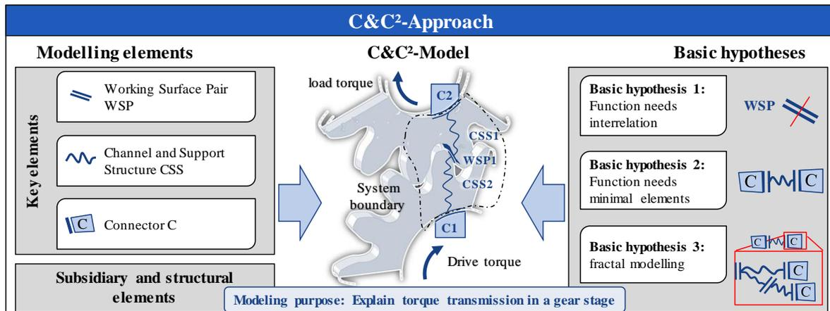
Figure 1. Overview of the C&C<sup>2</sup>-Approach and its elements (Matthiesen et al., 2018)
