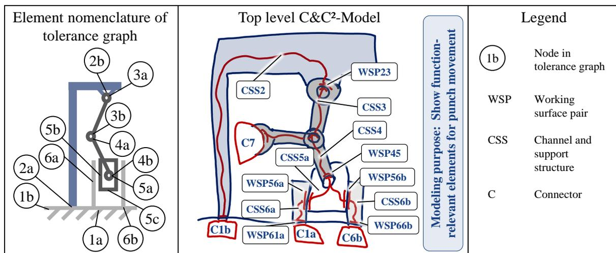
Figure 5. Top level models of the tolerance graph and C&C<sup>2</sup>-Approach
