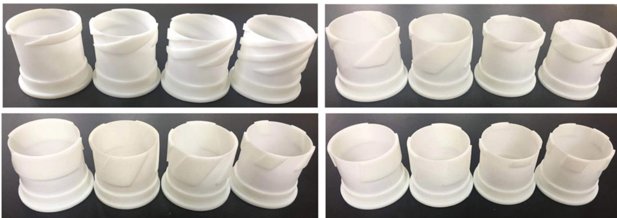
Fig. 6. Swirlers produced by 3D print technology.
