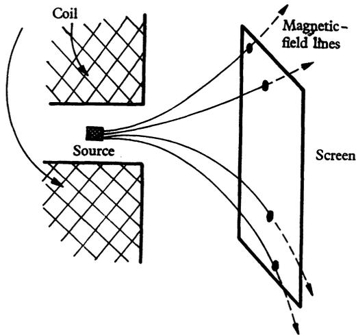
Fig. 3. Plasmoid source placed near the end of a coil. Spots are observed at a screen which indicates that the beam is shredded into streamers along the magnetic field.
