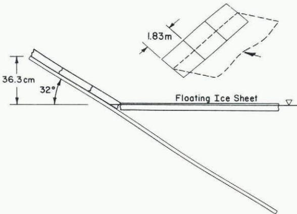
Fig.2. Sketch showing the freeboard and slope of the beach used in experiments 1, 2, 7 and 8.
