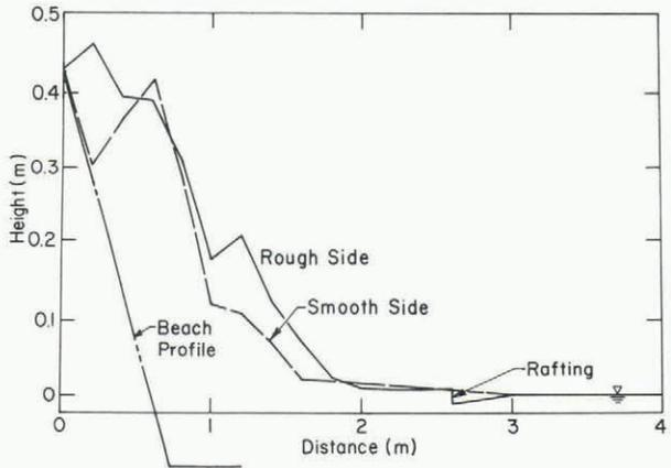
Fig.10. Profiles of the ice pile-up in experiment 12.
