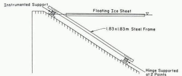
Fig.1. Sketch of steel frame 1.83 m wide.
