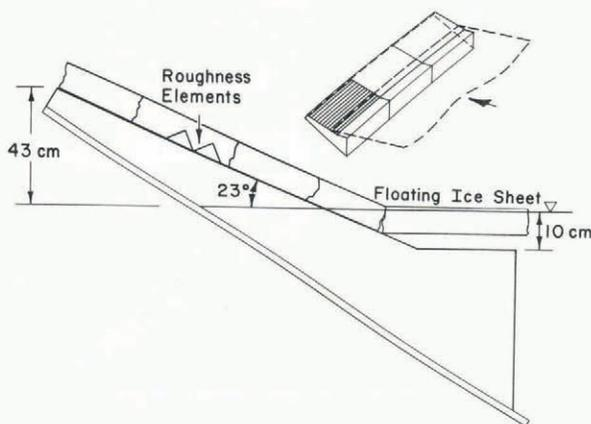
Fig. 5. Sketch of the beach used in experiment 5. The left segment of the beach is made rough by triangular wooden pieces.
