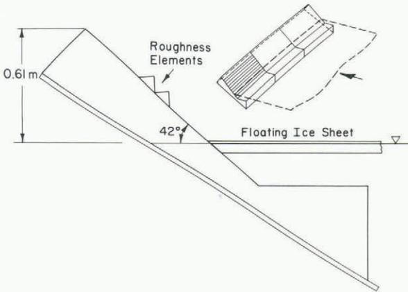
Fig.8. Sketch of the beach used in experiment 11. The left segment of the beach is rough.
