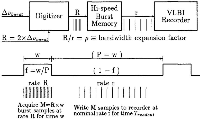
Fig. 1. BM acquisition system schematic and timing.
