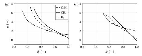
FIGURE 27. Evolution of  $a = \partial (S_L/\overline{S}_L)/\partial (\phi/\overline{\phi})$  as a function of the equivalence ratio  $\phi$  for propane/air (dashed lines), methane/air (solid lines) and hydrogen/air (dashed dotted lines) mixtures injected at T = 300 K and p = 1 bar (a) and p = 10 bar (b).
