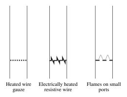
FIGURE 3. Examples of tubes in which self-sustained pressure oscillations are driven by heat addition.
