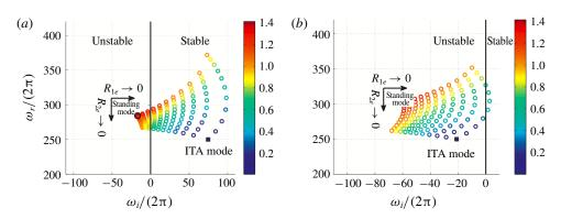
FIGURE 14. Trajectories of ITA modes for a toy model similar to figure 6 when the reflection coefficients of the inlet and outlet vary (Hoeijmakers *et al.* 2014). (a) Stable ITA mode  $(G(\omega_r) \leq G_c)$ . (b) Unstable ITA mode  $(G(\omega_r) \geq G_c)$ . The colour scale corresponds to the value of  $(R_1^2 + R_2^2)^{1/2}$  and measures the separation from a perfectly anechoic system.
