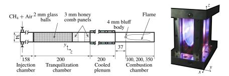
FIGURE 18. INTRIG set-up used at IMFT laboratory to study coupling between intrinsic and acoustic modes. The length of the combustion chamber can be fixed to 0.10, 0.20 or 0.35 m. The flame occupies a large fraction of the combustion chamber (Miguel-Brebion *et al.* 2016).
