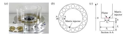
FIGURE 24. (a) MICCA annular combustor equipped with matrix laminar injectors. (b) Top view of showing the 16 matrix injectors. (c) Cut A-A view with the main dimensions. Adapted from Bourgouin et al. (2015).
