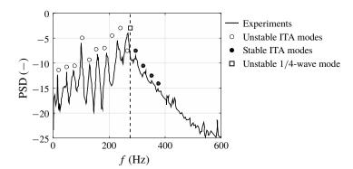
FIGURE 20. Pressure spectrum recorded in the INTRIG set-up quipped with an uncooled bluff body and a short combustion chamber l = 0.10 m. Adapted from Miguel-Brebion (2017).
