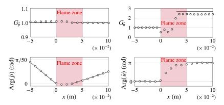
FIGURE 15. First ITA mode structure for the configuration of figure 6 (Courtine *et al.* 2014). Solid line: theory (4.9) and (4.10). Symbols: DNS.
