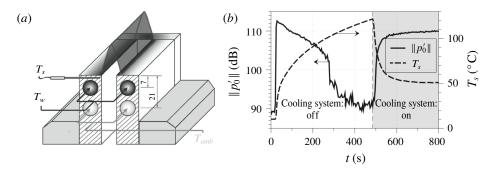
FIGURE 30. Effects of wall temperature on a laminar premixed dihedral flame Mejia *et al.* (2014). (a) Flame stabilized on a water-cooled slot. (b) Evolution of pressure oscillations and slot wall temperature versus time. The cooling system is started at t = 490 s.
