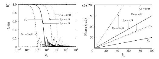
FIGURE 28. Gain (a) and phase (b) of the filters  $F_A$  and  $F_m$  as function of the dimensionless wavenumber  $k_*$  for different flame angle values  $\alpha = \pi/16$ ,  $\pi/8$ ,  $\pi/4$  and  $3\pi/8$ .  $k_*/\omega_* = (H/L)^2 = \cos^2 \alpha$ .
