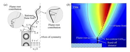
FIGURE 31. (a) The two mechanisms contributing to the FTF of an inverted V-flame stabilized on a slot (Cuquel *et al.* 2013a; Mejia *et al.* 2014). (b) Visualization of the stand-off distance between flame holder and flame root (Mejia *et al.* 2014).
