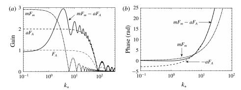
FIGURE 29. Gain (a) and phase (b) of the heat release rate response of a methane–air dihedral flame submitted to equivalence ratio oscillations in a homogeneous flow field;  $\bar{v} = 1 \text{ m s}^{-1}$ ,  $\bar{S}_L = 0.26 \text{ m s}^{-1}$ , H/L = 0.97.
