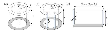
FIGURE 21. (a) Annular combustor system. The distance between the inner and outer cylinders forming the sidewalls is small compared to the mean radius  $d \ll (R_i + R_e)/2$ . (b) The annular combustor is unwrapped by cutting the geometry by an axial plane. (c) The equivalent rectangular combustor has a width  $\mathcal{P} = \pi(R_i + R_e)$ , its length is equal to that of the initial annular system. The depth is equal to the distance between the inner and outer cylinders  $d = R_e - R_i$ .
