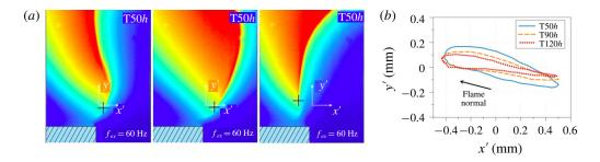
FIGURE 32. (a) Visualization of the flame movements for an inverted V-flame submitted to a 60 Hz forcing with a flame-holder temperature of 50 °C. The + symbol marks the flame root. (b) The trajectories of the flame root are displayed for three different temperatures of the flame holder (50, 90 and 150 °C) (Mejia et al. 2014).
