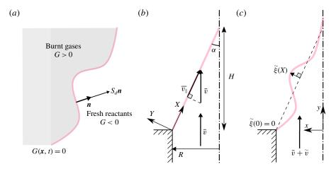
FIGURE 26. (a) Flame sheet G=0 separating fresh reactants form burnt gases. Steady (b) and perturbed (c) dihedral flame stabilized on a two-dimensional slit of half-width R. Here  $\alpha$ , flame angle; H, flame height; L, flame length;  $\bar{v}$ , mean axial flow velocity; and  $\bar{v}_{\parallel} = \bar{v} \cos \alpha$ , component of the mean axial flow velocity parallel to the flame front.
