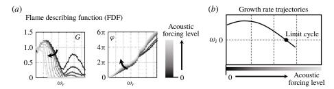
FIGURE 2. (a) Typical evolution of the gain G and phase lag  $\varphi$  of a flame describing function (FDF) as the acoustic forcing level increases. (b) Growth rate  $\omega_i$  of an unstable mode as a function of the acoustic forcing level leading to a limit cycle.
