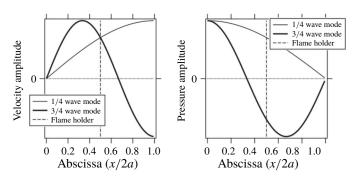
FIGURE 7. The structure of the 1/4 and 3/4 wave modes in the model of figure 6.
