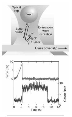
Figure. A combined optical trapping and fluorescence experiment to unzip DNA. (a) Schematic of the experimental geometry; (b) simultaneous measurements of the force required to rupture (top trace) and the fluorescence (bottom trace). The dye unquenched upon rupture and then later bleached. Courtesy Journal of Biology **2** (6)(2003); http://jbiol.com/content/2/1/6.
