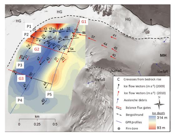
**Fig. 3.** Plan-view QuickBird satellite image of KPB showing firn-core location, crevasses on the inside bend of the glacier, surface ice-flow velocity vectors (m a<sup>-1</sup>) from 2009 and 2010, flux gates (red dotted lines, G1–G3) and ice depth contours extrapolated from GPR profiles (blue lines). The eastern depths of gate G3 (black dotted line) were interpolated for flux calculations.
