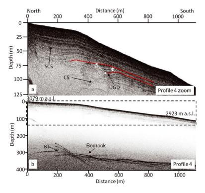
**Fig. 9.** Axial center-line 100 MHz GPR profile 4 of KPB showing: (a) zoom of upper 125 m and (b) full depth profile with zoom section outlined by dashed line. SCS overlies complex strata (CS), strata that dip up-glacier (UGD) and significant strata thickness variations (white arrows). A strong bedrock horizon and bow-tie reflections (BT) suggest overdeepening in the full profile.
