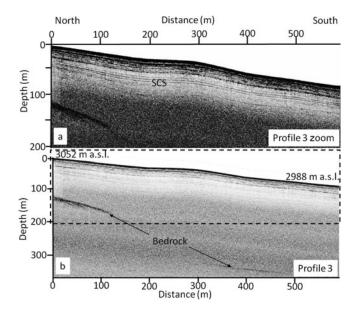
**Fig. 8.** Axial western 100 MHz GPR profile 3 of KPB showing: (a) SCS in upper 100 m zoomed section and (b) intermittent bedrock horizon in full profile. Zoom section is outlined by dashed line. Minimal variations in stratigraphy thickness or signs of deformation are present.
