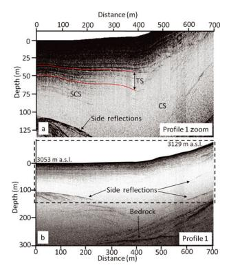
**Fig. 6.** 100 MHz GPR profile 1 within KPB showing: (a) zoom of upper 130 m with thickening strata (TS), SCS and CS, west to east, and (b) full depth profile with the black dashed line representing zoomed region in (a). A strong bottom horizon and side reflections are also visible in (b). Side reflections occur because of the GPR profile's close proximity to the valley headwall. The deepest internal horizon is interpreted as bedrock.
