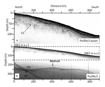
**Fig. 10.** Axial eastern 100 MHz GPR profile 5 of KPB showing: (a) complex strata (CS) in upper  $\sim$ 90 m depth and (b) varied bed topography with overdeepening (OD) suggested by bow-tie reflections (BT) at 100 m distance, where ice plunges from MH into KPB and at 850 m where ice flows out of KPB to the south. Dashed line represents zoomed section in (a).
