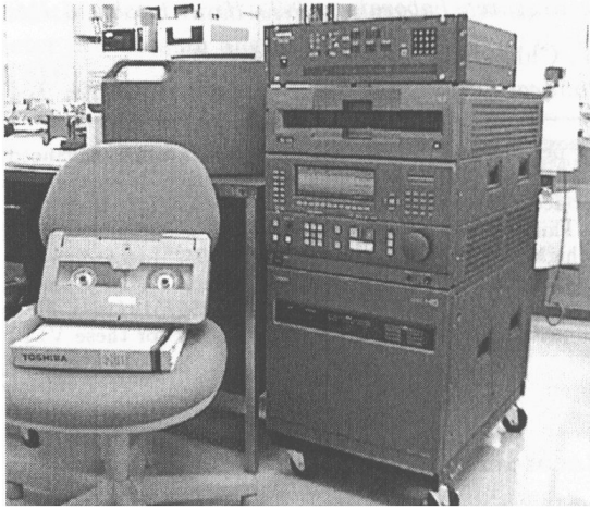
Figure 1. GBR-1000 transport and processor under experiment. Upper small unit is the DRA-1000 interface. Cassette size of the D-6 is same to the former K4(ID-1). The Data packing density is 4 times higher. components.
