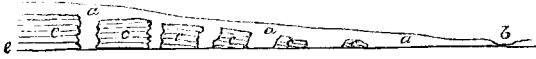
Fig. 6. a , Drift clay filling up fissures in Ragstone beds, c c ; b , Bed of the Medway.
