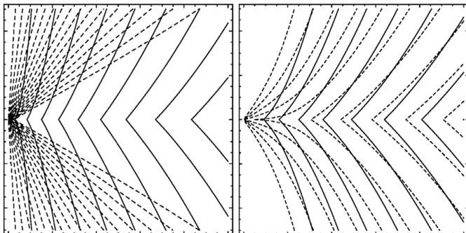
**Figure 4.** Magnetic field lines. The box on the left has dimensions 10 AU on each side, while the box on the right has dimensions 100 AU on each side. The dashed lines represent the flux-freezing model ( $\eta_0 = 0$ ) while the solid lines show the same field lines for  $\eta_0 = 1$ . The second core has just formed and is on the left axis midplane.
