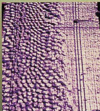
SNOM image (above) and topographic image (right) of eye tissue were acquired simultaneously by Aurora.
