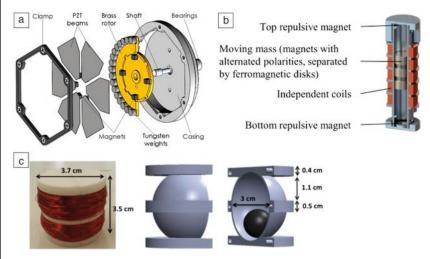
Figure 4. Wearable inertial energy-harvester architectures: (a) eccentric rotor,<sup>32</sup> (b) linear slide,<sup>39</sup> and (c) spherical magnet in spherical cavity.<sup>41</sup> Note: PZT, lead zirconate titanate, Pb(Zr<sub>0.52</sub>Ti<sub>0.48</sub>)O<sub>3</sub>.
