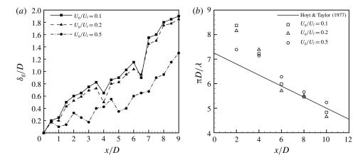
FIGURE 7. The growth of gas boundary layer thickness ( $\delta_g$ ) along the axis (a); and comparison of the dimensionless wavenumber,  $\pi D/\lambda$ , obtained from the simulations, with the experimental data of Hoyt & Taylor (1977) (b).
