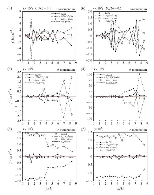
FIGURE 34. (Colour online) Comparison of the terms in the axial momentum equation (a,b), azimuthal momentum equation (c,d) and radial momentum equation (e,f), for case 1 (a,c,e) and case 3 (b,d,f);  $t^* = 11.5$ .
