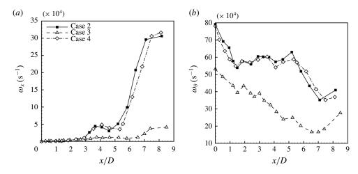
FIGURE 36. Axial distribution of  $\omega_x$  (a) and  $\omega_{\theta}$  (b) for cases 2, 3 and 4, at  $t^* = 11.5$ .
