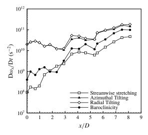
FIGURE 37. Contributions of streamwise vortex stretching, azimuthal vortex tilting, radial vortex tilting and baroclinicity to the generation of  $\omega_x$  at the jet surface for case 4;  $t^* = 11.5$ .
