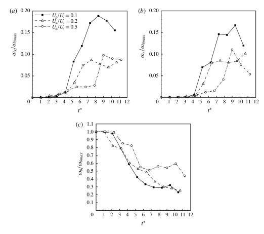
FIGURE 23. Kinematic variation of the normalized  $\omega_x$  (a);  $\omega_r$  (b); and  $\omega_\theta$  (c) for different velocity ratios.
