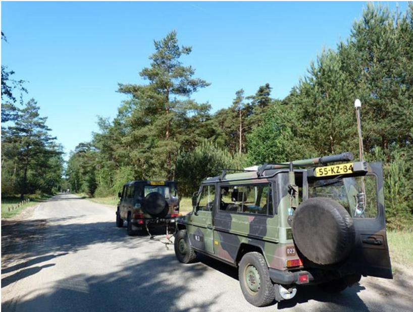
Figure 7. MB with E-field measurement set-up pulled by second MB in the first survey.
