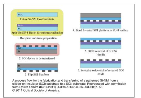
to transfer electronic and photonic devices without compromising structural integrity and functionality. The researchers describe their fabrication protocols in the January 1st issue of *Optics Letters* (DOI:10.1364/
