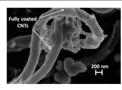
Scanning electron micrograph of multiwalled carbon nanotubes coated with BaTiO<sub>3</sub>.
