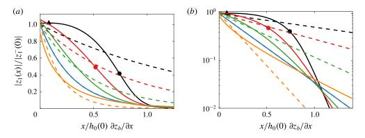
FIGURE 8. (Colour online) (a) Admittance of the tide for the case where the depth varies along the river (bold) and for the case where the depth remains constant along the river (dashed); inflexion points are indicated by dots, maxima by chevrons; (b) the logarithmic y-axis reveals the inversion of the stage-amplitude relation in the asymptotic reach; scenarios as in figure 7(a).
