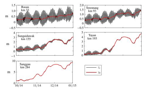
FIGURE 3. (Colour online) Time series of the surface elevation  $z_s$  (black) and its tidal average  $z_0$  (red) at five gauging stations along the Kapuas River;  $z_0$  is determined by low pass filtering with a cutoff period of one tidal cycle so that the subtidal variation over the spring-neap cycle remains.
