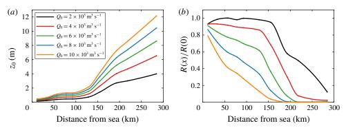
FIGURE 4. (Colour online) (a) Observed tidally averaged water level and (b) admittance of tidal range along the Kapuas River at different river discharges.
