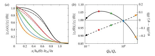
FIGURE 12. (Colour online) (a) Admittance of the combined incoming and reflected waves  $(|z_1(x)|/|z_1^-(0)|, \text{ solid})$  and only of the upstream travelling wave  $(|z_1^-(x)|/|z_1^-(0)|, \text{ dash-dotted})$  along the river. (b) amplitude (solid) and phase (dashed) of the combined wave with respect to the incoming wave at the river mouth, depending on the river discharge. Scenarios as in figure 8.
