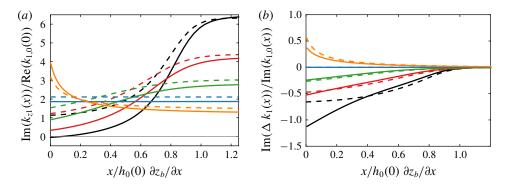
FIGURE 10. (Colour online) (a) Imaginary (dashed) and real (solid) parts of the wavenumber  $z_1$ , corresponding to the rate of damping and phase change, respectively; critical damping occurs at  $\text{Im}(k_{1z}) = 0$ . (b) Relative strength of convergence compared to that of gravity and friction ( $\text{Im}(\Delta k_1/k_{1,0})$ , solid) and its approximation by (3.23*a*) (dashed), critical damping occurs at -1; scenarios correspond to those in figure 8.
