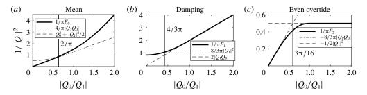
FIGURE 5. Magnitudes of the frequency components of the friction term ((3.8a)-(3.8c), bold), depending on the relative strength of river and tidal flow  $(|Q_0|/|Q_1|)$ , as well as their low flow asymptotes  $(|Q_0|/|Q_1| \rightarrow 0, \text{ dash-dotted})$  and high flow asymptotes  $(|Q_0|/|Q_1| \rightarrow \infty, \text{ dashed})$ . Note that the discharge scale is identical to the velocity scale as  $|u_0|/|u_1| = |Q_0|/|Q_1|$ .
