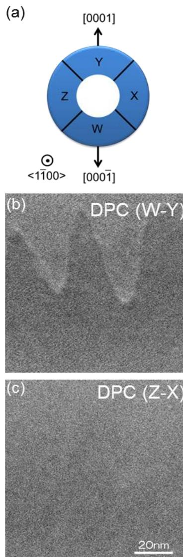
Fig. 2. (a) Schematic illustration showing the relationship between the crystallographic orientation of LiTaO<sub>3</sub> and the four detector segments. (b)(c) DPC STEM images of a 180 degree domain wall.
