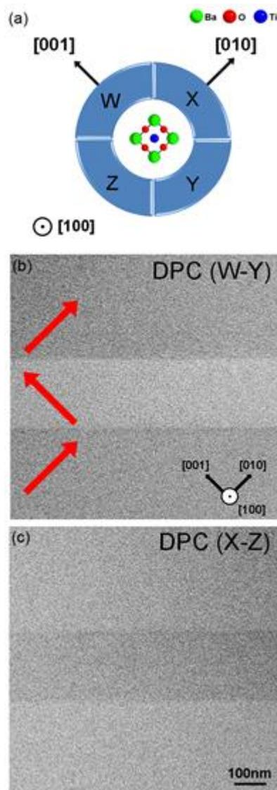
Fig. 1. (a) Schematic illustration showing the relationship between the crystallographic orientation of BaTiO<sub>3</sub> and the four detector segments. (b)(c) DPC STEM images of 90 degree domain structure.
