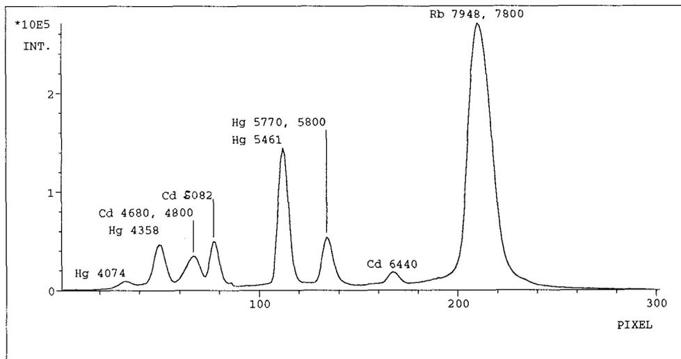
**Figure 4:** Hg-Cd-Rb calibration spectrum.
