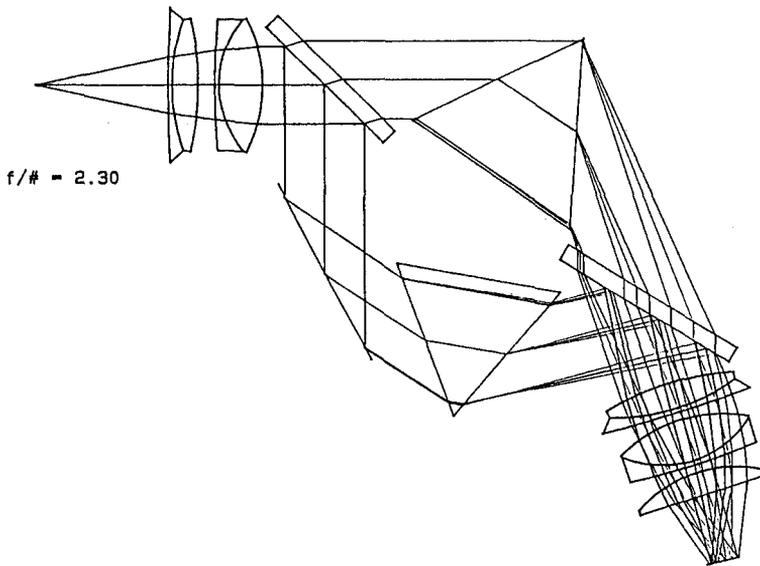
**Figure 3:** Double beam prism spectrograph.
