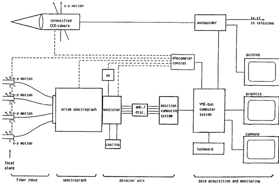
**Figure 1:** Block diagram of the 4-Channel-Spectral-Photometer.
