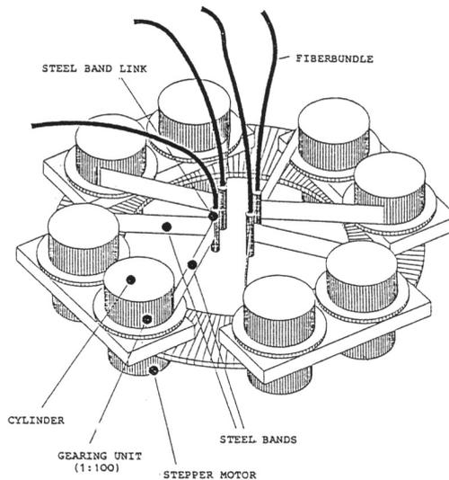
**Figure 2:** Fiber positioning unit.
