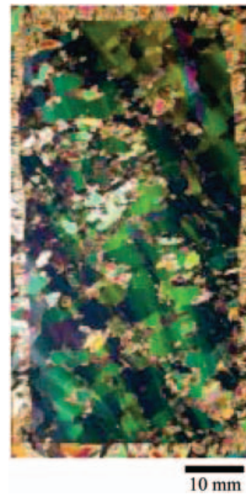
Fig. 7. Photography of a vertical thin section from 2593 m depth after deformation at 19% strain.
