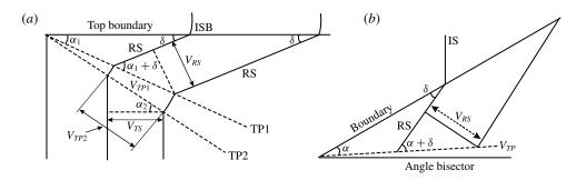
FIGURE 13. Sketch of angles of the top horizontal boundary with the refracted shock front ( $\delta$ ) and with the trajectories of the two triple points ( $\alpha_1$  and  $\alpha_2$ ).  $V_T$ , the transmitted shock speed;  $V_R$ , the refracted shock speed;  $V_{TP}$ , the triple point speed.
