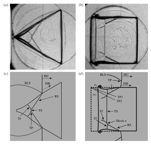
FIGURE 9. Wave patterns of a shock interacting with the forward-triangle at  $t = 90 \ \mu s$ (*a*) and with the square at  $t = 91 \ \mu s$  (*b*):  $\alpha_1$  and  $\alpha_2$ , the angles of the trajectories of the two triple points with the initial horizontal interface;  $\delta$ , the angle of the refracted shock front with the initial horizontal interface. ISB and ISC are the incident shock along and away from the interface, respectively.
