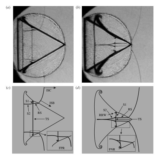
FIGURE 10. Wave patterns of a shock interacting with the backward-triangle at  $t = 82 \ \mu s$ (a) and  $t = 177 \ \mu s$  (b). The symbols are the same as those in figure 9.
