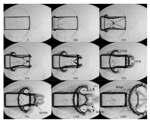
FIGURE 4. Experimental schlieren images of the shocked SF<sub>6</sub> streamwise-rectangle inhomogeneity. M = 1.18. SDVR, second downstream vortex pair. Other symbols and the description of the wave patterns are the same as those in figure 3.
