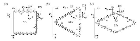
FIGURE 16. Sketch maps of the vorticity generation on the boundaries for the square (*a*), forward-triangle (*b*) and diamond (*c*).  $\nabla p$ , pressure gradient caused by the incident shock;  $\nabla p'$ , pressure gradient caused by the diffracted shock.
