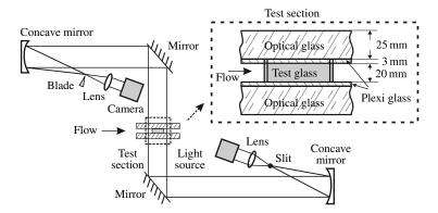
FIGURE 2. Schematic diagram of the schlieren system.
