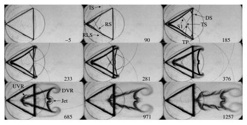
FIGURE 6. Experimental schlieren images of the shocked SF<sub>6</sub> forward-triangle inhomogeneity. M = 1.19. RLS, reflected shock. Other symbols and the description of the wave patterns are the same as those in figure 3.
