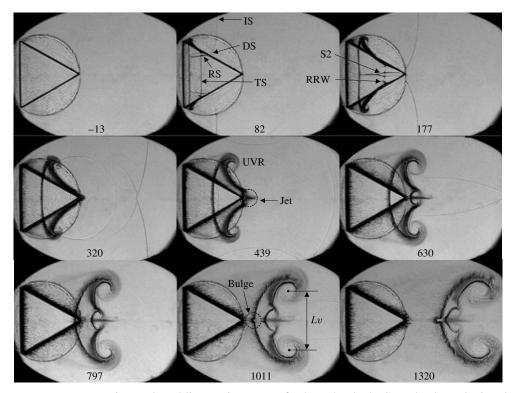
FIGURE 7. Experimental schlieren images of the shocked SF<sub>6</sub> backward-triangle inhomogeneity. M = 1.19. RRW, reflected rarefaction waves. Other symbols and the description of the wave patterns are the same as those in figure 3.
