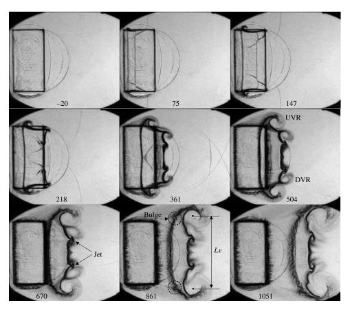
FIGURE 5. Experimental schlieren images of the shocked SF<sub>6</sub> transverse-rectangle inhomogeneity. M = 1.19. The symbols and the description of the wave patterns are the same as those in figure 3.
