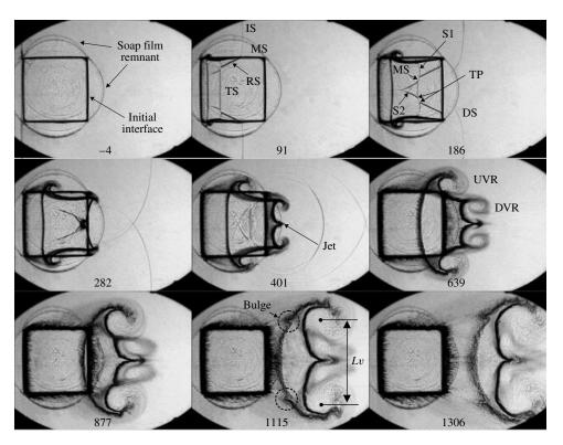
FIGURE 3. Experimental schlieren images of the shocked SF<sub>6</sub> square inhomogeneity. M = 1.17. IS, incident shock; TS, transmitted shock; RS, refracted shock; TP, triple point; MS, Mach stem; DS, diffracted shock; S1 and S2 are the products of the interaction between the TS and RS. UVR, upstream vortex pair; DVR, downstream vortex pair; Lv, vortex spacing. The numbers indicate the time after the shock impact and the unit is  $\mu$ s.
