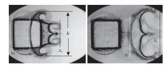
FIGURE 15. Schematic sketch of the distances measured for SF<sub>6</sub> square inhomogeneity.
