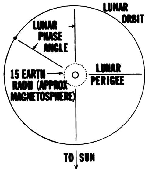
**FIGURE 1. COORDINATE SYSTEM USED FOR EJECTA ORBIT CALCULATIONS**
