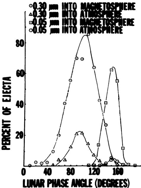
FIGURE 2. PERCENT OF EJECTA INTERCEPTED BY EARTH'S MAGNETOSPHERE AND ATMOSPHERE
