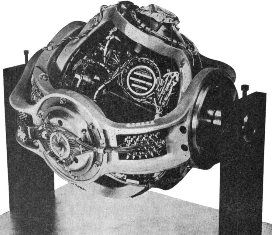
*Fig. 1. Miniature platform for inertial guidance.*
