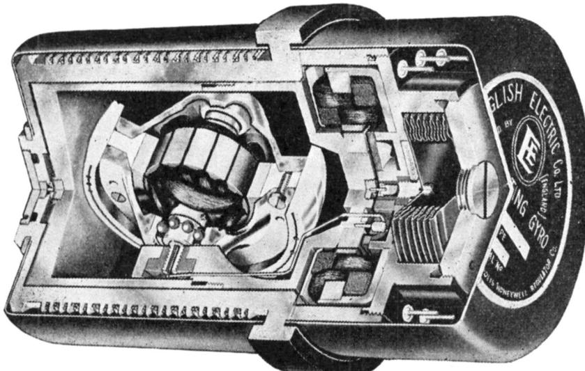
*Fig. 3. Miniature rate-integrating gyroscope.*
