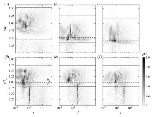
Figure 7. Compensated one-dimensional spectra of the streamwise velocity fluctuations along the vertical span at the centre of the FOV  $x/h_c = 10.25$  for (a) F1, (b) F3 and (c) F5 seagrass scenarios, and (d) R1, (e) R3 and (f) R5 rigid canopy cases. Dashed lines indicate the canopy top  $(h_d)$ , and dotted lines denote the location of  $z_1$  and  $z_2$ .
