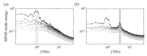
Figure 10. Spectral proper orthogonal decomposition (SPOD) spectra of the rigid R5 case of the flow field (a) above and (b) within the canopy, with the darkest (black) line being the first SPOD mode and the lighter lines the subsequent SPOD modes.
