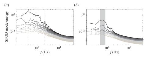
Figure 12. SPOD spectra of the seagrass, F5 case, of the flow field (*a*) above and (*b*) within the canopy, with the darkest (black) line being the first SPOD mode and the lighter lines the subsequent SPOD modes.
