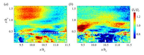
Figure 17. Conditional average of sweep to ejection ratio during the F5 flexible canopy (*a*) downward motion phase and (*b*) upward motion phase.
