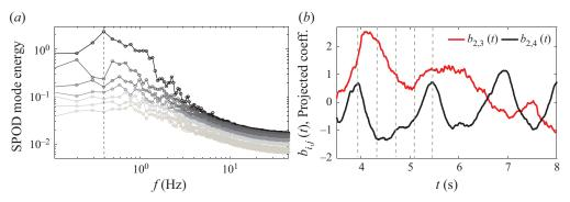
Figure 14. (a) Full flow field SPOD spectrum on the seagrass F5 case. The darkest to lighter lines indicate the progression from the first to the fourth SPOD modes; (b) projected SPOD mode coefficients,  $b_{i,j}(t)$  for the *i*th mode of *j* frequency.
