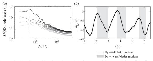
Figure 16. (a) SPOD spectra form the quadrant analysis of the seagrass F5 case. The darkest to lighter lines indicate the progression from the first to the fourth SPOD modes; (b) projected SPOD mode coefficients,  $b_{1,4}(t)$  for the first mode of 0.6 Hz.
