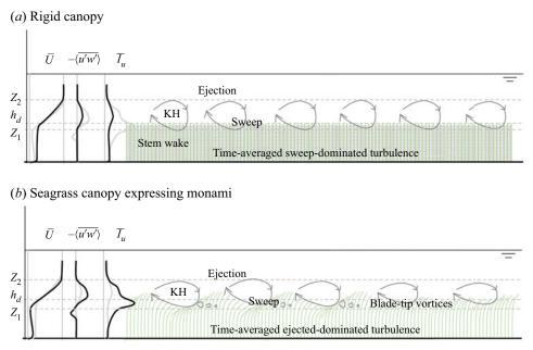
Figure 18. Schematic summary of flow processes associated with (a) rigid canopy and (b) flexible canopy based on  $Re \sim 10^5$ .
