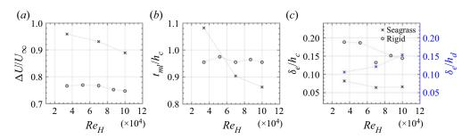
Figure 5. (a) Velocity change within canopy, (b) mixing layer thickness, (c) vortex penetration depth relative to the undeflected canopy height (left axis) and vortex penetration relative to the deflected canopy height (right axis). Data are shown for both the flexible seagrass and rigid canopy.
