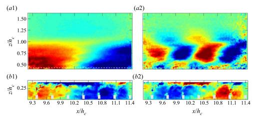
Figure 13. Spatial organisation of the first SPOD modes above the canopy at f = (a1) 0.4 Hz and (a2) 2.25 Hz; and within the canopy at f = (b1) 0.6 Hz and (b2) 0.68 Hz.
