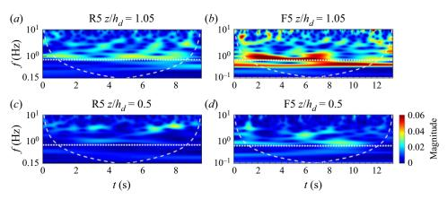
Figure 8. Wavelet representation of the streamwise velocity within and immediately above the flexible (F5) and rigid (R5) canopies at  $Re = 1.1 \times 10^5$ . (a) R5,  $z/h_d = 1.05$ , (b) F5,  $z/h_d = 1.05$ , (c) R5,  $z/h_d = 0.5$ , (d) F5,  $z/h_d = 0.5$ . White dashed lines indicate the cone of influence, and horizontal dotted lines mark  $f_{KH}$ .
