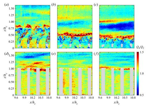
Figure 6. Ratio of total contribution of sweep (Q4) and ejection (Q2) events for the seagrass scenarios (a) F1, (b) F3, (c) F5 and rigid canopy cases (d) R1, (e) R3, (f) R5. Dashed white lines indicate the mean canopy height.
