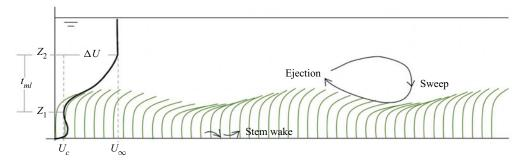
Figure 1. Basic features common in aquatic vegetation canopies. Here,  $t_{ml}$  represents the mixing layer and  $\Delta U$  indicates the associated bulk velocity difference. Stem wake flow may not occur in fully flexible stems as discussed below.
