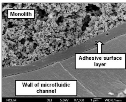
Figure 1. Scanning electron micrograph showing the cross section of a porous polymer monolith inside a delaminated microchip fabricated in a cyclic olefin copolymer (COC).
