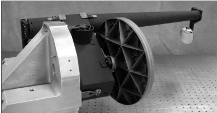
Figure 1. The SiC telescope developed by SSG Precision Optronics for the geosynchronous imaging Fourier transform spectrometer (GIFTS) space flight mission.
