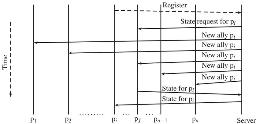
Fig. 5. Joining a non-empty universe.
