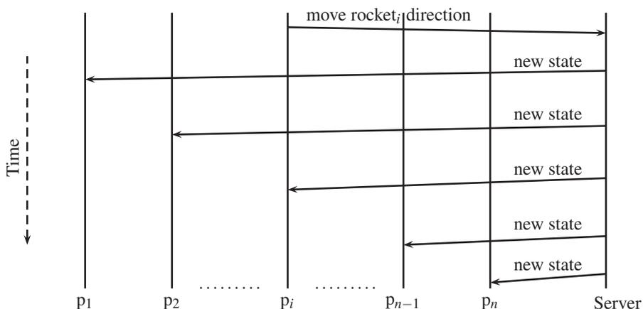
Fig. 12. Version 2 protocol diagram for a rocket move.
