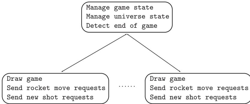
Fig. 11. Components for thick-server version of multiplayer Aliens Attack.
