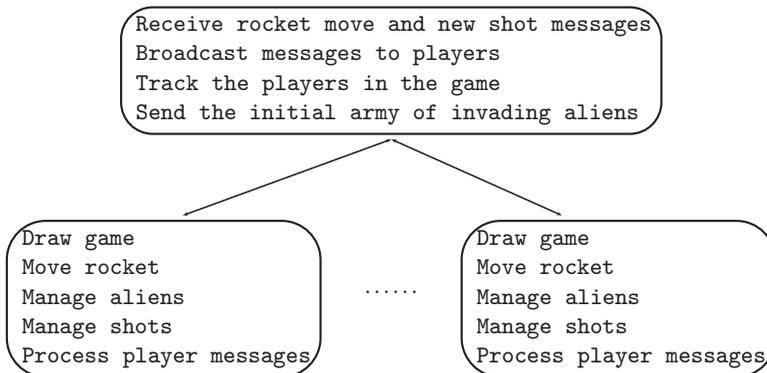
Fig. 2. Components for thin-server version of multiplayer Aliens Attack.
