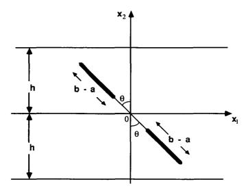
FIGURE 1. A pair of arbitrarily-oriented coplanar cracks in an anisotropic slab.
