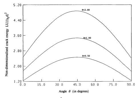
FIGURE 3. Variations of  $LU/(s_0d)^2$  with  $\theta$  for a/d = 0.25, R = 1.334 (titanium) and h/d = 2.50, 3.50 and 4.50 as well as h/d tending to infinity.
