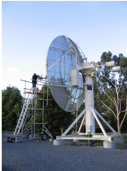
Figure 3. 6-m radio telescope (Auckland) used in the first Trans-Tasman (New Zealand–Australia) VLBI observations in 2005.
