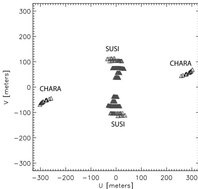
**Figure 3.** Baseline and position angle coverage of Spica from the CHARA/FLUOR and SUSI interferometers mapped on the U-V plane. CHARA's long east-west projected baselines at  $K$ -band have equivalent resolving power to SUSI's longest baselines at  $700 \text{ nm}$ .
