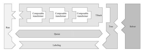
Fig. 14. The components of a CP model with composable search transformers and how they fit together.
