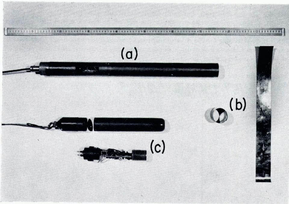
Fig. 2. (a) Marker implanter with (b) one coiled and one uncoiled marker. (c) Detector instrument with electronic contents. The scale is one meter long.
