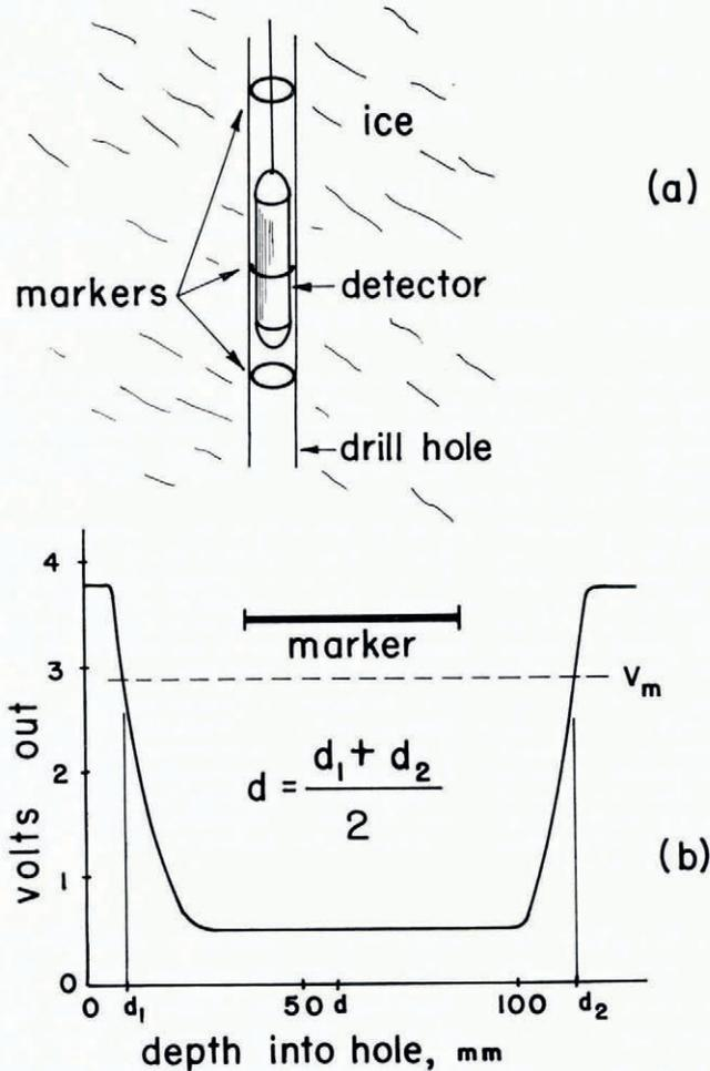
Fig. 1. (a) Sketch of detector instrument located in drill hole with markers in place. (b) Electrical output in vicinity of marker.
