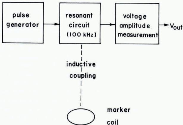
Fig. 3. Block diagram of detector electronics.
