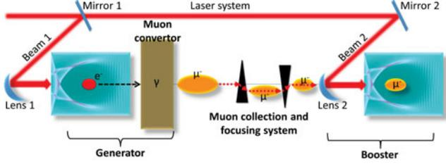
**Figure 1.** All-optical ‘Generator and Booster’ scheme of muon source. Muons are first generated by the Bethe–Heitler process, the ‘Generator’, via high-energy photons from Bremsstrahlung radiation of laser wakefield accelerated electrons interacting with high  $Z$  materials. After a proper collection and focusing system, muons are boosted by another laser wakefield, the ‘Booster’.
