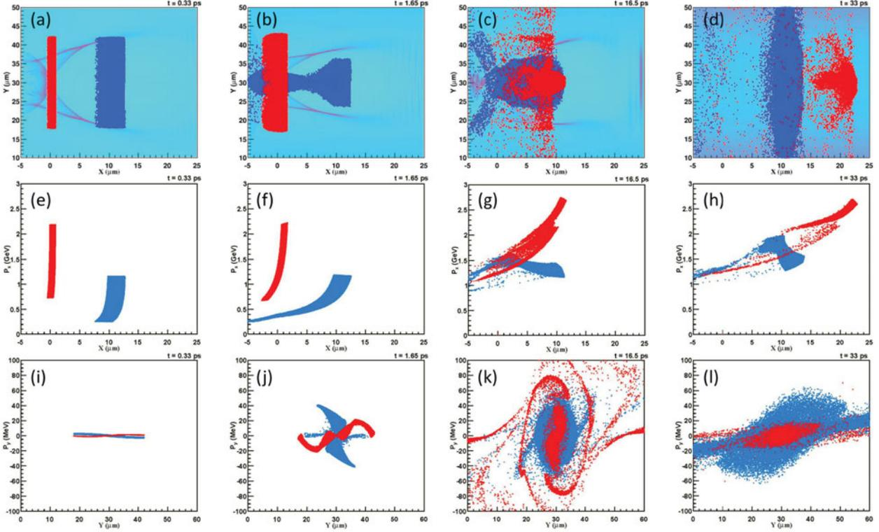
**Figure 4.** The snapshots of the acceleration processes of forward (red dots) and backward (blue dots) muons from the two-dimensional PIC simulations in Figure 2 at (a)  $t = 0.33$  ps, (b) 1.65 ps, (c) 16.5 ps and (d) 33 ps. (e)–(h) The  $x$ - $p_x$  and (i)–(l)  $y$ - $p_y$  phase spaces of forward (red dots) and backward (blue dots) muons at the four snapshots are also shown, respectively.
