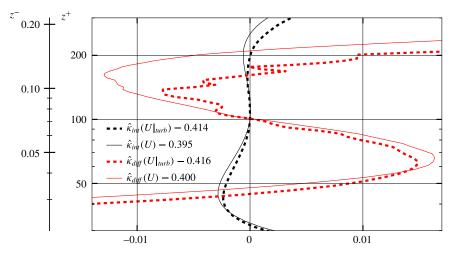
FIGURE 7. (Colour online) Deviation of the estimates for the von Kármán constant based on its value at  $z^- = 100$  (cf. table 2). Estimates of  $\hat{\kappa}_{int}$  based on the integral formulation (5.2*a*) are shown in black, estimates of  $\hat{\kappa}_{diff}$  based on the differential formulation in red. Thick, dashed lines are based on averages conditioned to turbulent patches  $(U|_{turb})$  and thin solid lines show conventional averages (U).
