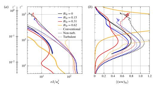
FIGURE 10. (Colour online) Viscous dissipation rate of TKE (a) and TKE (b) conditioned to turbulent and non-turbulent regions of the flow. The secondary vertical axis applies to the neutrally stratified case only.
