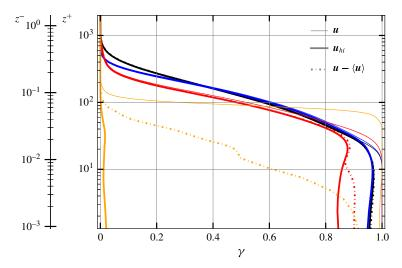
FIGURE 5. (Colour online) Intermittency factor  $\gamma$  with a threshold vorticity  $\omega_0 = \tilde{\omega}$  calculated from high-pass filtered field (thick solid:  $\mathscr{F}^+_{\delta}$ ; thick dash-dotted: Reynolds' decomposition) and unfiltered field (thin solid). Colours indicate the stratification as in figure 4. The secondary vertical axis applies to the neutrally stratified case only.
