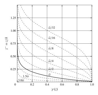
FIGURE 3. Intermittency factor versus height for case ri00 varying the intermittency threshold  $\omega_0$  in the range  $\tilde{\omega}/32 \leq \omega_0 \leq 3\tilde{\omega}$  with  $\tilde{\omega}$  as defined in (4.2).
