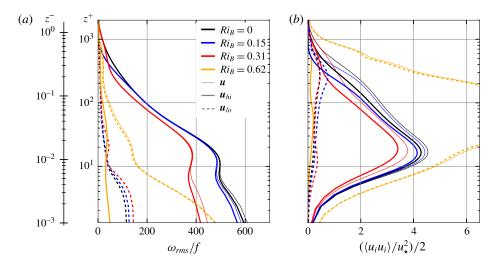
FIGURE 4. (Colour online) Vertical profiles of the vorticity root mean square (a) and TKE (b) of the unfiltered (thin solid), high-pass (thick, solid) and low-pass (thick dashed) filtered fields for case ri00 (black), ri15 (blue), ri31 (red) and ri62 (orange).
