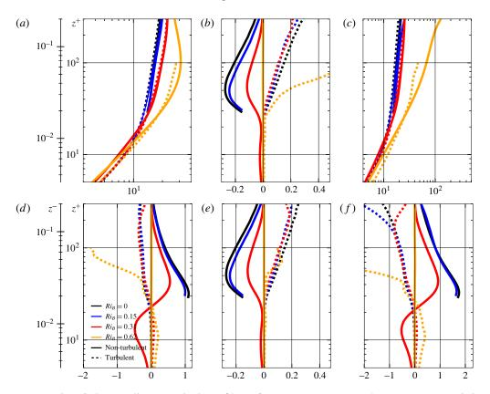
FIGURE 9. (Colour online) Vertical profiles of U, W, B (a-c), and  $U_{hi}$ ,  $W_{hi}$ ,  $B_{hi}$  (d-f) conditioned to non-turbulent and turbulent sub-volumes of the flow. The lines are drawn if the area fraction contributing to a partition at a given level exceeds 1 %. The secondary vertical axis applies to the neutrally stratified case only.
