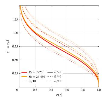
FIGURE 11. (Colour online) Intermittency factor versus height for the case ri00 and the lower-*Re* case re\_low with Re = 7725 where the intermittency threshold is varied by a factor of 8 (note that the variation in *Re* from 7725 to 26450 corresponds to a variation of  $\nu$  by a factor of 4).
