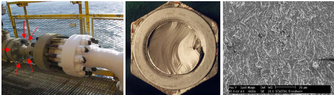
Fig. 1 High cycle fatigue; beach marks and transgranular fracture morphology.
