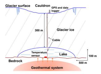
**Fig. 3.** Schematic drawing of the western Skaftá cauldron showing the  $\sim$ 300 m thick floating ice shelf penetrated by a drillhole into the  $\sim$ 100 m deep subglacial lake and the scientific instruments deployed in the lake and on the glacier surface in the campaign in 2006. Note that the vertical scale is exaggerated five-fold.
