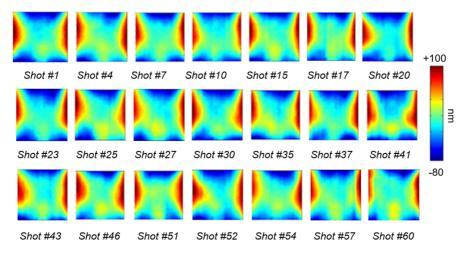
**Figure 3.** Spatial distribution of the amplified transmitted wavefront along a 1 h sequence at 1 shot per minute, flow rate of 29 L/min, as measured with the wavefront analyzer. A great stability of the wavefront is obtained with an RMS of less than 0.08% for the PV value over the whole sequence (see Table 1). Some vertical lines can be observed on some shots (e.g., shot #43), induced by the coolant flow.
