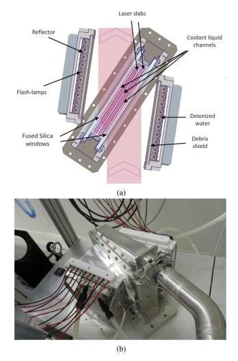
**Figure 1.** (a) Schematic of the liquid-cooled split-slab amplifier cell. The pink vertical line represents the laser beam. (b) Photo of the assembled amplifier.
