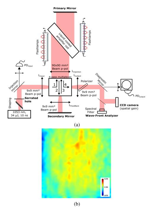
Figure 2. (a) Experimental setup used to characterize the amplifier in a four-pass configuration. The gain is measured using photo-diodes (PDs). Spatial distribution of gain is measured on a CCD camera. Wavefront distortion is measured with an HASO wavefront analyzer. (b) Single-pass gain distribution of the clear aperture of 90 mm  $\times$  90 mm (1 shot/min, 29 L/min). A gain average of 1.151 is obtained with a standard deviation of 0.013 over the 90 mm  $\times$  90 mm area.
