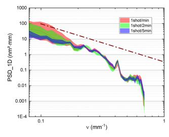
**Figure 4.** One-dimensional PSD over the (1-10 mm) range calculated from the wavefront measurements. Each envelope represents the minimum-to-maximum PSD variation along a 1 h sequence at a flow rate of 29 L/min for repetition rates of 1 shot/min, 1 shot/2 min and 1 shot/5 min, respectively. The purple dashed line is a guide to the eye representing a typical PSD specification for ICF laser slabs<sup>[17,18]</sup>.
