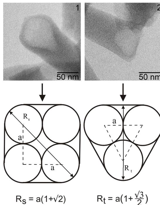
Figure 2. The analysis of the cross-sectional shapes of two SWNT ropes selected in Fig. 1c. The TEM image magnifications of the square- (1) and triangular- (2) cross-section areas are shown on top. Below are presented their schematic model approximation together with, placed in the bottom, the formulas relating square- ( $R_s$ ) and triangular- ( $R_t$ ) cross-section diagonals of the corresponding SWNT ropes to the SWNT bundle diameter ( $a$ ).
