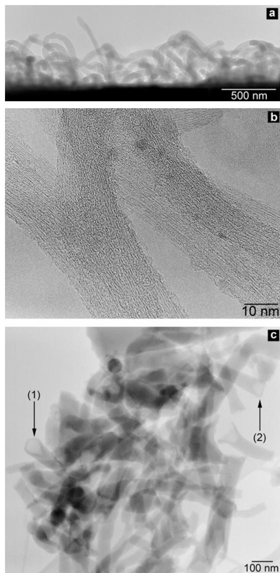
Figure 1. (a) Cross-sectional TEM image of the SWNT sample after its exposure to atomic deuterium for 60 min., (b) and (c), high- and low-magnification TEM images of the SWNT material scraped from the sample presented in (a), respectively. Low-magnification TEM image (c) shows thick ropes of bundles characterised by square- (1) and triangular-cross-sections (2).
