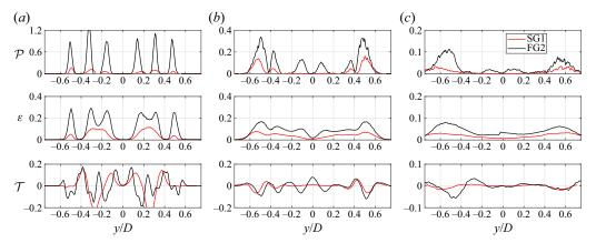
Figure 10. Production, dissipation and transport terms in the turbulent kinetic energy (3.1) for the fractal FG2 and single square SG1 grids. Data are measured at (a)  $x/x^* = 0.1$ , (b)  $x/x^* = 0.24$ , i.e. corresponding to the peak of turbulent kinetic energy, and (c)  $x/x^* = 0.5$ . Data are normalized with respect to  $U_b^3/D$ .
