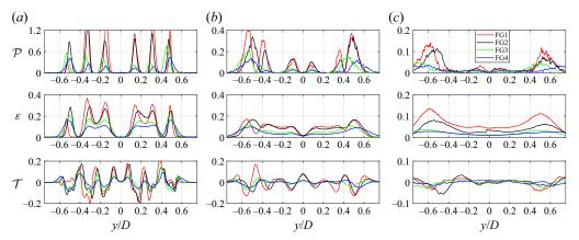
Figure 11. Production, dissipation and transport terms in the turbulent kinetic energy (3.1) for the four investigated FGs. Data are measured at (a)  $x/x^* = 0.1$ , (b)  $x/x^* = 0.24$ , i.e. corresponding to the peak of turbulent kinetic energy, and (c)  $x/x^* = 0.5$ . Data are normalized with respect to  $U_h^3/D$ .
