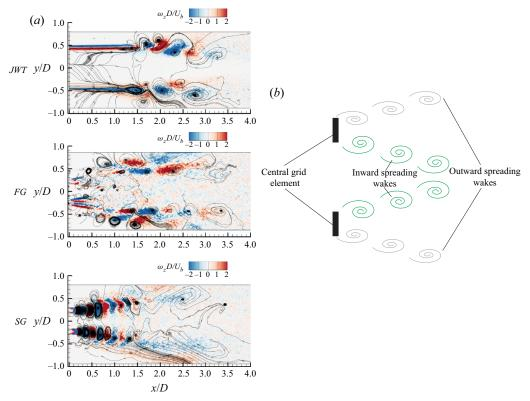
Figure 12. (a) Contour representation of the instantaneous out-of-plane fluctuating vorticity component  $\omega_z D/U_b$  with overlaid streamlines. Three different inlet conditions are considered: JWT, FG2 and SG1. The instantaneous realization is obtained as a low-order reconstruction considering only the first 10 most energetic modes. (b) Schematic description of the inward and outward spreading wake.
