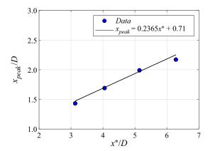
Figure 9. Location of the maximum in the  $u'/U_b$  profiles for the four investigated FGs,  $x_{peak}$ , as a function of the wake interaction length scale  $x^*$ . Data are normalized with respect to the jet diameter D.
