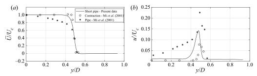
Figure 2. (a) Mean streamwise velocity and (b) r.m.s. of the streamwise velocity profiles measured at x/D = 0.05 and normalized with respect to the centreline velocity value  $U_c$ . Data are compared with the measurements of Mi *et al.* (2001) taken at the same Reynolds number (16 000) for different inlet conditions, namely a contraction and a pipe nozzle.
