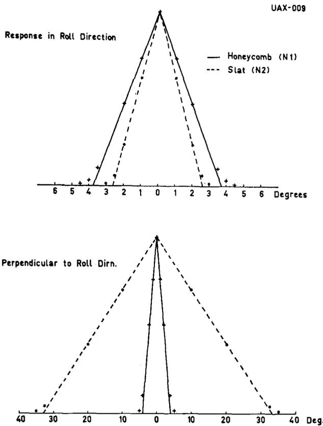
Figure 3. Measured collimator responses of the N1 and N2 detectors.
