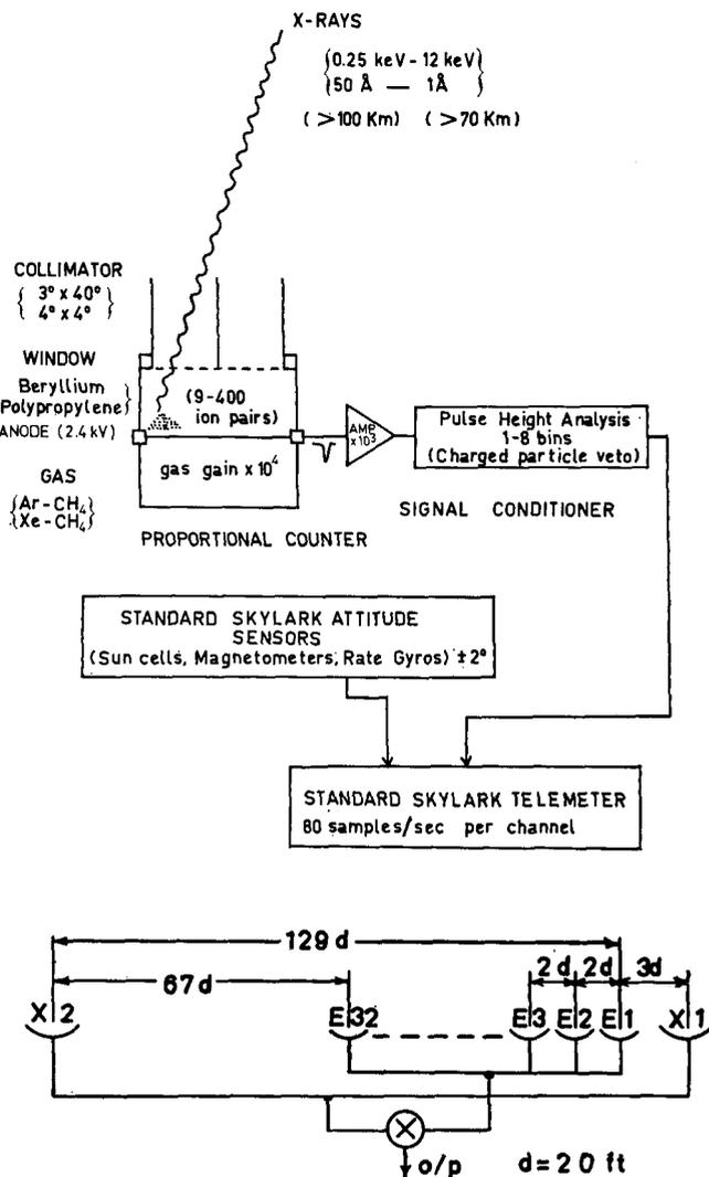
Figure 2. Basic UAT Skylark experiment, illustrating typical detector and rocket limitations.
