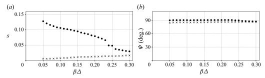
**Figure 6.** (a) Curvilinear position of the maximum magnitude of the optimal roughness and response as a function of  $\beta\Delta$ . (b) Local  $\Psi$  angle of the optimal roughness and response at the location of the maximum magnitude. The values related to the optimal roughness and responses are respectively depicted by crosses and circles.
