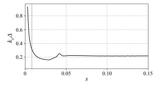
**Figure 5.** Curvilinear evolution of  $k_s \Delta$  of the optimal roughness with  $\beta \Delta = 0.11$ . The location of the maximum magnitude of the optimal roughness is shown (green vertical dashed line).
