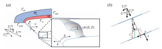
**Figure 1.** (a) Schematic of the mesh and flow configuration with a zoom on a roughness of any shape. (b) Angles and coordinate systems are indicated. An external streamline is illustrated in green. The blue lines correspond to the leading/trailing edges.
