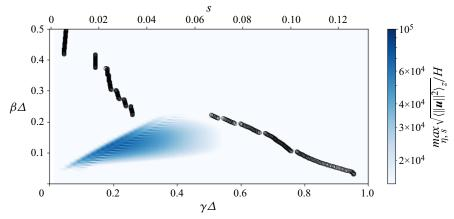
**Figure 11.** Representation, according to  $\beta\Delta$  and  $\gamma\Delta$ , of  $\max_{\eta,s}(\sqrt{\langle ||\mathbf{u}||^2\rangle_z})/H$ . The curvilinear location where the maximum of the function for optimal perturbations is reached is plotted in black circles with respect to the top axis.
