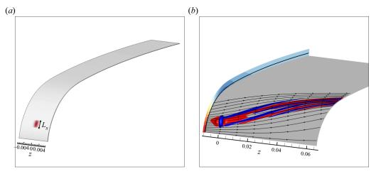
**Figure 9.** (a) Three-dimensional representation of the localised roughness h(s,z)/H with  $s_0 = 0.008 \approx 82\Delta$ ,  $L_s/\Delta = 20.6$ ,  $L_z/\Delta = 10.3$ . (b) Spatial structure of the corresponding response calculated by solving the LNSE, with the same representation as in figure 3.
