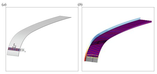
Figure 7. (a) Shape h(s,z)/H of the square wave roughness with  $L_z/\Delta = 2\pi/0.11 \approx 57.1$  and  $L_s/\Delta = 2\pi/0.32 \approx 19.6$  and localised at  $s_0 = 0.008$ . The positive and negative values are represented in red and blue, respectively. (b) Associated response calculated solving the LNSE with the same representation as figure 3. The yellow ellipse indicates the area where a difference with the response calculated using the approximation (5.4) occurs.
