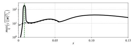
**Figure 10.** Curvilinear evolution of  $\max_{\eta}(\sqrt{\langle ||\mathbf{u}||^2\rangle_z})$  of the response computed using (5.7) (dashed line) and the exact (3.11) (solid line). The location of the centre of the roughness is shown by the green vertical dashed line.
