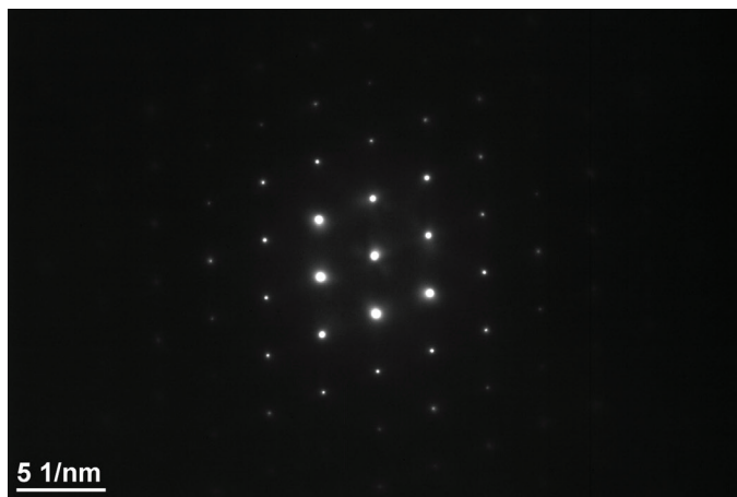
Figure 1: Si [011] SAED single crystal pattern showing that the beam block is not required when the intensity of the spots is uniformly distributed.
